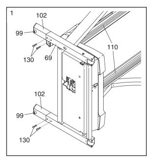
Attach four Base Pads (99) to the base of the Uprights (69) with four 1" Screws (148). Note: One replacement Base Pad may be included. Use the Base Pad to replace any Base Pad that becomes worn.
